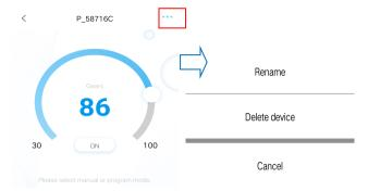
The user can change the pump name as want for easy management. The user can delete the current pump also. But when want to add the pump again, need to reconfigure the network.
