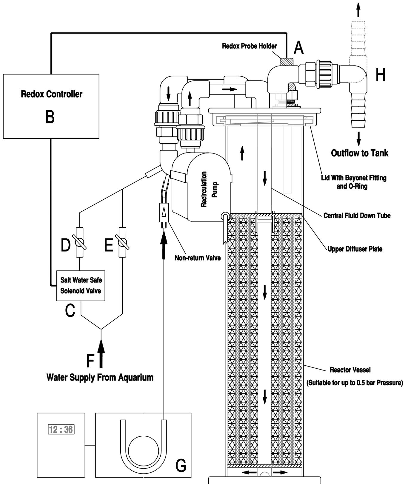
Nitrate Fluid Supply Using a Timer & Peristaltic Pump
