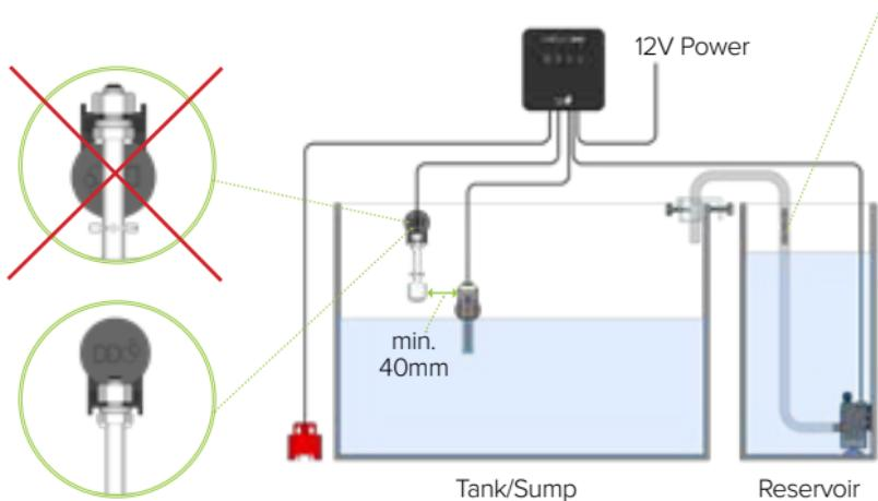
The Advanced ATO controller needs to be fixed in a suitable location away from splashing water and areas of high humidity. It should not be mounted directly above open water. Do not connect power to the ATO unit until setup is complete.
